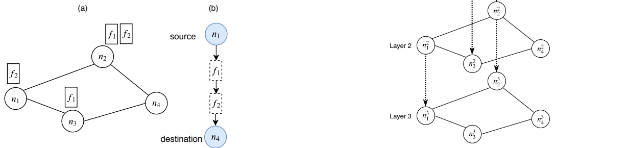
Figure: (Left): (a) A network substrate along with the permissible NFs on each network element, and (b) the logical topology of a service request. (Right) The auxiliary network transformation for the problem input.
